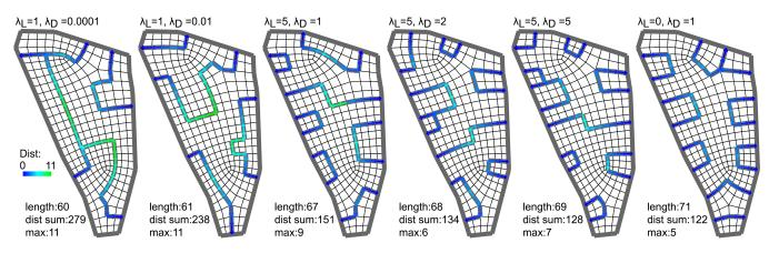
**Figure 5:** Optimization results with changing  $\lambda_L$  (to minimize network lengths) versus  $\lambda_D$  (to minimize travel distances). A larger  $\lambda_L$  leads to shorter network lengths but longer travel distances, while a larger  $\lambda_D$  leads to the opposite.
