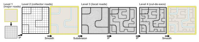
Figure 3: Pipeline. For each sub-region, as determined by the input major roads, we generate layouts in three levels of decreasing coverage ranges. For each level, a rough street network is first generated by the IP-based approach (shown in gray). Afterwards, the geometry of the generated street network is refined by a smoothing process. Dead-ends are typically allowed only at the last level.
