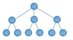
Figure 3: A sample index tree. Root:  $G_1^0 = \{1, 2, 3, 4, 5, 6, 7, 8\}$ . Depth 1:  $G_1^1 = \{1, 2\}, G_2^1 = \{3, 4, 5, 6\}, G_3^1 = \{7, 8\}$ . Depth 2:  $G_1^2 = \{1\}, G_2^2 = \{2\}, G_3^2 = \{3, 4, 5\}, G_4^2 = \{6\}, G_5^2 = \{7\}, G_6^2 = \{8\}$ .
