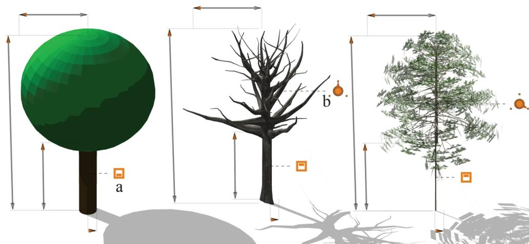
Figure 18: The boolean handle (a) is used to switch between a schematic (left) and a realistic tree (middle & right). When the scope containing the realistic tree is created, a range handle (middle, b) is shown, which can be used to change the tree type (right).
