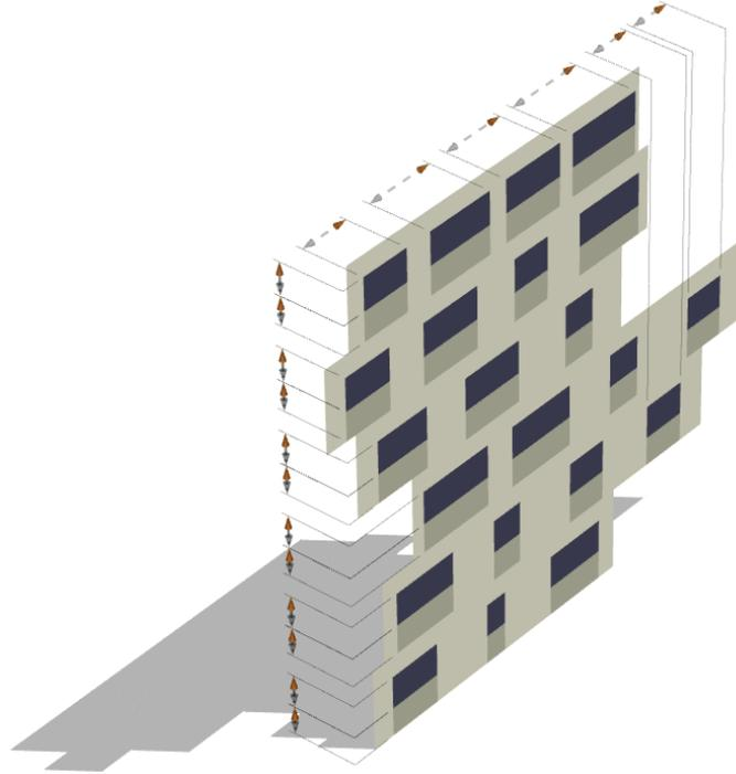
Figure 14: A facade with 3 parameters dimensioned using chain lines: windowsill height, window width, and window height. The width parameter is multiplied by a random value to obtain various window sizes, so an indirect chain dimension line is used, indicated by dashed gray dimension lines (top). Note how the snap guide on the left supports two parameters on a single line.
