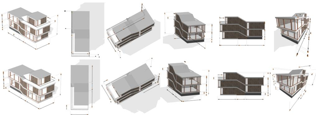
Figure 19: **Helix House**. Top: world space static dimension line positions. Bottom: our system creates dimension lines that are visible, usable, and consistent with design principles at a wide range of camera positions and fields of view.
