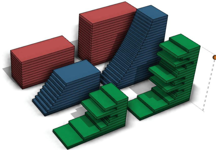
Figure 17: These buildings are parameterized by total floor area. We wish to position the dimension line as shown, to control this parameter. In the red case there is a linear relationship between the line and parameter value. In the green and blue cases there is a non-linear relationship. **Indirect handles** provide an appropriate line length and editing behavior. Note the stippled dimension line, and author specified spherical decoration.
