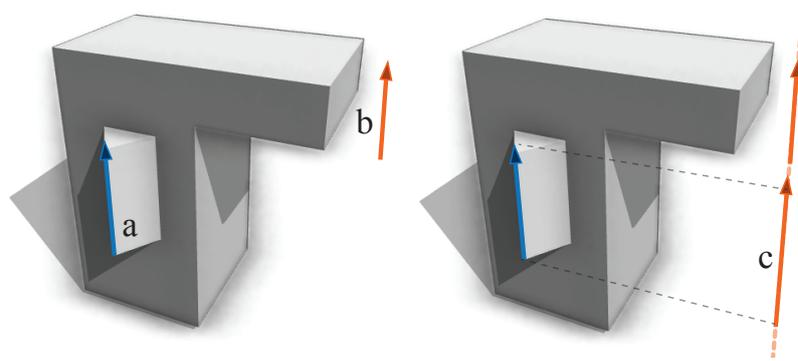
Figure 8: Left: A final line (b) in  $G_{\text{snap}}$ , and a baseline (a) which we are processing. Right: we find the guide line (dashed orange) on the same plane as (a), and use it to position the new candidate line (c).
