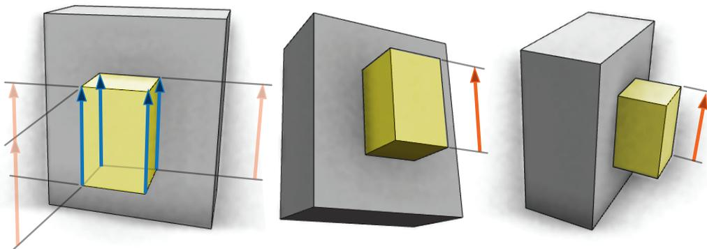
Figure 3: To create an interactive dimension line on a parametric model, the author assigns a parameter to a scope (yellow). Per-frame, our system then computes candidate lines (left) and selects, using a scoring function, a final dimension line for a given view direction (middle, right).
