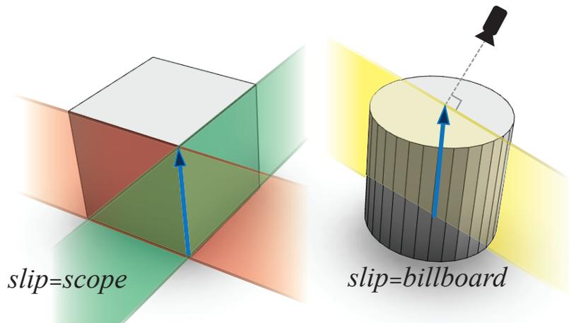
Figure 6: Left: **getScopePlanes** in Algorithm 1 aligns two scope aligned planes through the base line. Right: **getBillboardPlanes** creates a single plane through the base line, oriented in the view direction.
