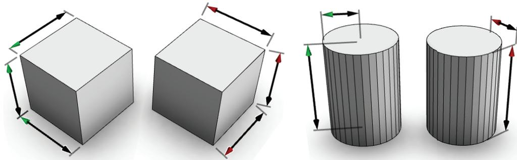
Figure 2: According to convention and standards, there are good (green) and bad (red) positions for dimension lines; see also the accompanying video.
