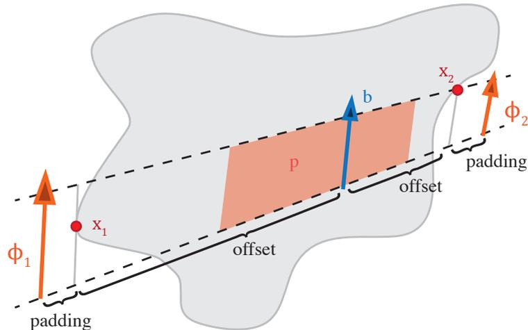
Figure 9: The geometric construction of candidate lines. Our goal is to compute the minimal translation of line ( $b$ ) over the plane ( $p$ ) so that the candidate lines can be placed without intersecting the model silhouette (gray shape). The final candidate lines ( $\phi_1$  and  $\phi_2$ ) are moved by an additional padding distance beyond their nearest intersections ( $x_1, x_2$ ).
