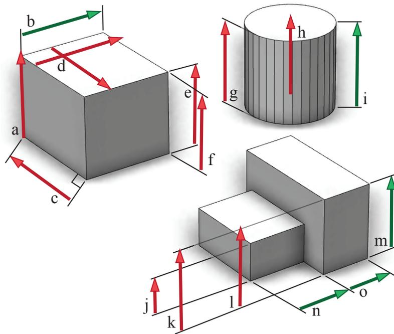
Figure 4: Examples of good (green) and bad (red) dimension lines illustrating the design principles of Subsection 3.1.
