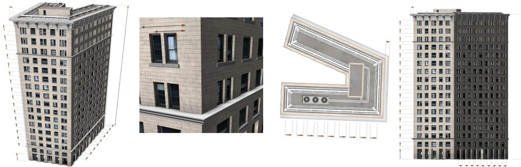
Figure 24: **Candler Building**, Georgia, USA. Left: a three quarters perspective view. Middle left: dimension lines are positioned inside the silhouette when zoomed in. Middle right: orthographic top view. Right: orthographic side view.
