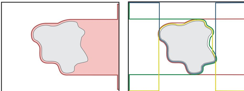
Figure 11: We compute four distance fields to approximate the silhouette of the model. One distance field is computed for each of the four viewport edges. Left: the distance field from the left boundary. Right: all four distance fields approximate the model's silhouette.
