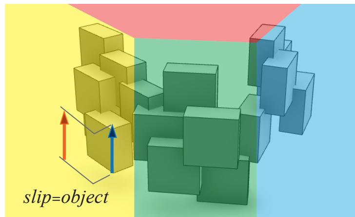
Figure 7:  $P_{\text{object}}$  defines a set of partially bounded global planes (red, green, yellow and light blue) aligned to the model's geometry; typically the planes will not pass through the base line's scope. A base line (blue arrow) finds a candidate position (orange arrow) on a plane (yellow).
