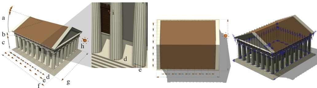
Figure 23: **Parthenon**, Athens, Greece. Left: as we zoom into the model, it becomes impossible to position dimension lines outside the silhouette. We see that dimension lines d (column spacing) and e (column radius) are positioned on their base lines. In addition short lines with a minimum display length (i) become visible. Also of note are the three chained dimension lines (def). Near right: orthographic top view. Far right: base line positions (blue).
