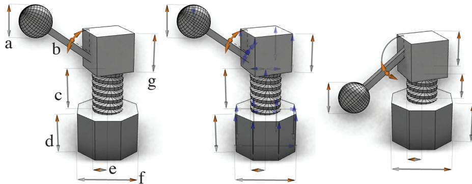
Figure 20: **Sprung Lever**. Left: a) type=spherical diametric, slip=billboard; b) rotational, none; c) linear center, billboard; d & g) linear contour, scope; e) radial, billboard; f) diametric, billboard. Middle: base lines (blue). Right: changing the configuration of the model causes the dimension lines to re-calculate their positions.
