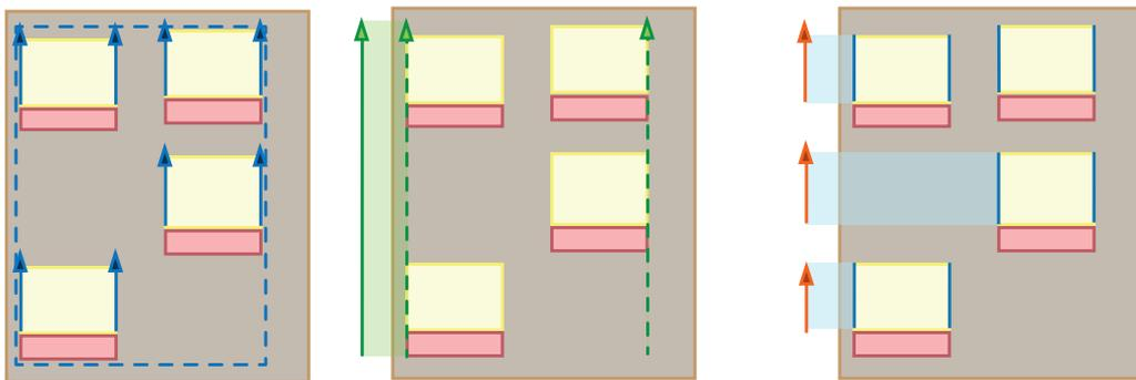
Figure 13: **Chained dimension lines** (red arrows) align final lines from the same parameter. The alignment is implemented by finding several candidate chain base lines (dashed green arrows), and then finding the most suitable, the **final chain line** (solid green arrow). Final dimension lines are projected onto this final chain line.
