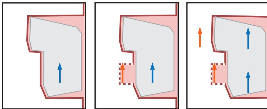
Figure 16: Left: the left distance field (red) for a model, and a base line (blue). Middle: the distance field after positioning the candidate line (orange). The winning line sets the boolean flag for the region it has updated (red dashed line). Right: this allows subsequent final dimension lines to be positioned avoiding existing final dimension lines.
