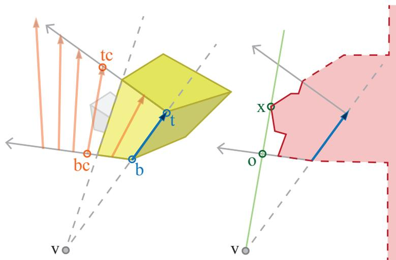
Figure 10: 2D screen space offset calculations. Left: due to the perspective projection to 2D screen space, base lines rotate and change length as they are offset in world space. Right: offset computation using a distance field (red dashed line) clipped to the extension and base lines (red solid line).
