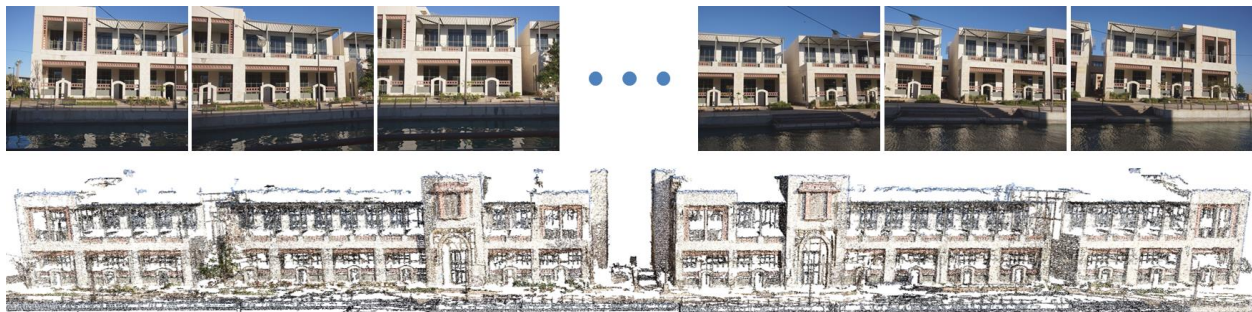
Figure 1: From a set of ground level images (top), we reconstructed a point cloud (bottom) that is used in the teaser example of our paper.
