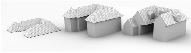
Fig. 32. Left: Straight skeleton; Middle: Straight Skeleton with angle changes; Right: Procedural extrusions
