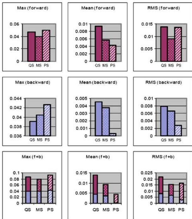
**Fig. 16.** Max, mean, and RMS error values for the wheel model simplifications of 318 triangles. Forward (original-to-simplified), backward (simplified-to-original), and forward plus backward errors are shown for Qslim (QS – left), memoryless simplification (MS – middle), and our method (PS – right)
