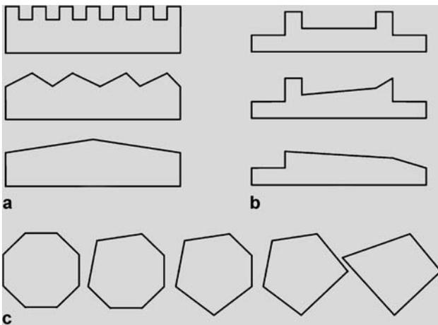
**Fig. 2a–c.** Problems with successive vertex merging. Small features merge into larger ones (a). In the window with frame (b) and the circle (c) some intermediate steps are intuitively not correct
