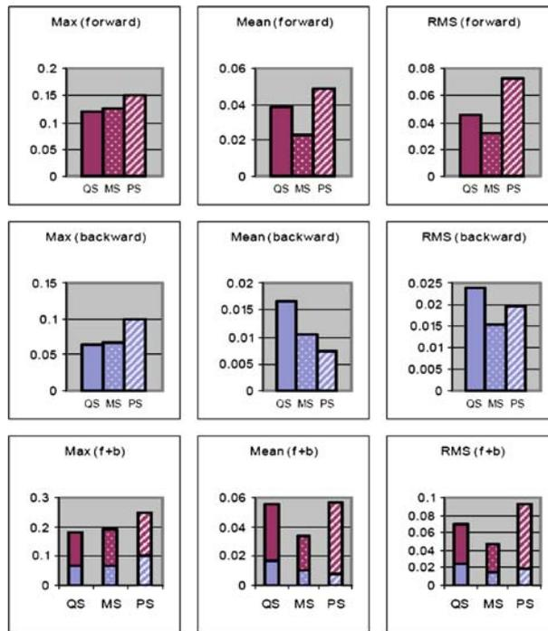
**Fig. 17.** Max, mean, and RMS error values for the wheel model simplifications of 76 triangles. Forward, backward, and forward plus backward errors are shown for Qslim (QS), memoryless simplification (MS), and our method (PS)
