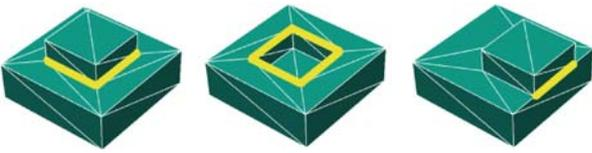
**Fig. 8.** Three edge types, highlighted in yellow. Left – concave. Middle – convex. Right – planar
