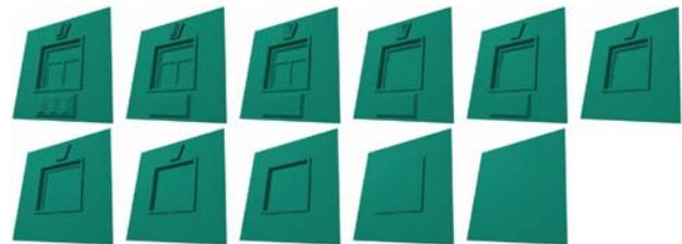
**Fig. 15.** A sequence of simplifications of a window model is automatically extracted with our algorithm. Entire features are removed per step, while the rest of the model is retained
