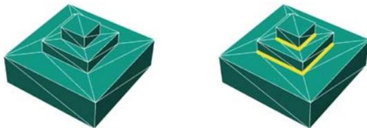
**Fig. 5.** A simple model (*left*) and two detected loops on the surface of the model shown in yellow (*right*). Not all possible loops are shown
