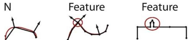
**Fig. 4a–c.** Three cases of mesh features. **a** Smooth surfaces: normals per vertex; the mesh is only seen as an approximation to the actual (smooth) surface; differential geometry applies. **b** Smooth surfaces with features: these are smooth surfaces that have sharp edges and corners. The edges and corners are called features. **c** Plane-dominant objects: the mesh is the actual geometry; normals are per polygon and not per vertex. A feature is a larger connected part of the mesh
