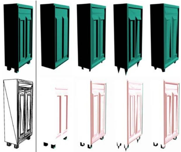
**Fig. 13.** *Top left*: the original armoire model with 476 polygons. *Bottom left*: wireframe of the original. *Top row*: selected simplifications using our algorithm (94 triangles), Qslim (94 triangles), memoryless simplification (94 triangles), and Maya (96 triangles) [25]. *Bottom row*: corresponding difference images (negative image) of the simplifications to the original
