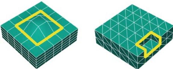
**Fig. 9.** A feature on a plane (*left*) and a feature on an edge (*right*)
