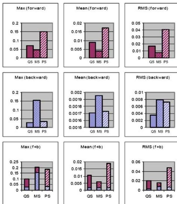
**Fig. 18.** Max, mean, and RMS error values for the armoire model simplifications of 94 triangles (from LOD 5 of 10). Forward, backward, and forward plus backward errors are shown for Qslim (QS), memoryless simplification (MS), and our method (PS)
