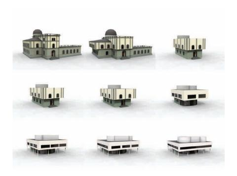
This animation demonstrates transformations of architectural design. The video shows buildings designed by two great architects, Gottfried Semper and Le Corbusier, and the emergence of new designs using a novel modeling system to compute design transformations. The modeling system, based on design grammars, captures the essence of architectural styles and computes their transformation.
