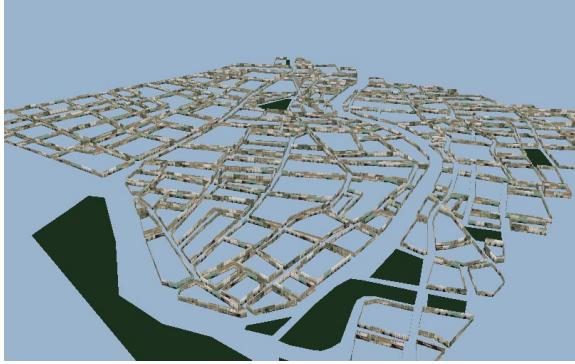
**Figure 9:** The figure shows the building fronts that are used as occluders in the urban walkthrough. The parks are shown as green textured polygons and are not used as occluders.
