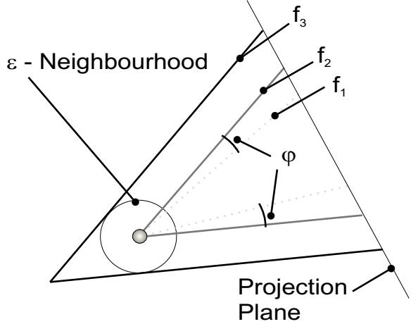
**Figure 6:** Adjusting the frustum for perspective projections. The original frustum  $f_1$  is made wider by an angle of  $\varphi$ . The resulting frustum  $f_2$  is then moved back to yield a frustum  $f_3$  tight on the  $\epsilon$ -neighborhood, to accommodate rotation and movement during the time  $t_\epsilon$ .
