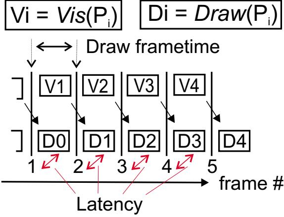
**Figure 2:** Parallelization in the traditional pipeline introduces latency and limits the time available for visibility. The figure shows where additional latency is introduced.
